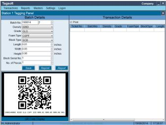
Tagging Software (Tagsoft) is application software for the weight capturing and printing label in the field of Foam, Plastics, Rubber, Foods and Wood productions. This software can be used to weigh all type of objects and print the *Barcode* or *QR Code* or *Plane labels*. It can transfer data to Cloud, Shared or Main server database in online and offline mode.
