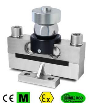
Double shear beam load cells particularly suitable for weighing weighbridges, dosage systems, tanks, silos, etc., complete with support and oscillating spherical joint. CE-M approved.
