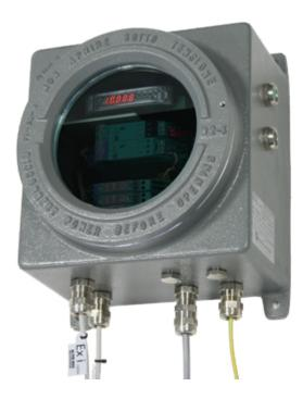
Box with Exd protection completed with weight indicator/transmitter, Zener barriers and intrinsically safe 4-20mA analog output. Fitted with 2 buttons for the main weighing operations with configurable functions, and two programmable electronic outputs for setpoints and levels management. Complete protection: ATEX II 2 (1) GD Ex d [ia Ga] IIC T6 Gb / Ex tb [ia Da] IIIC T85°C Db IP66.
