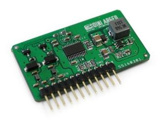
16 bit analogue output, in voltage or in current. Programmable as 0...5/0...10Vdc, 0...20/4...20mA through the **indicator** or through the PC with Dinitools. Particularly suitable for use with PLC's and in industrial environments.
